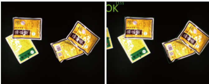
Distinguishing and positioning identification of the upper and lower stacked bags of seasoning.
